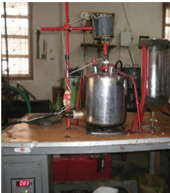
Figure 7. Photographic view of the biodiesel reactor (stirring and heating the raw oil, methanol, catalysts at 60°C).
